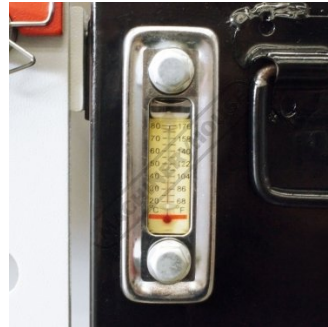
Hydraulic Oil Level Gauge
